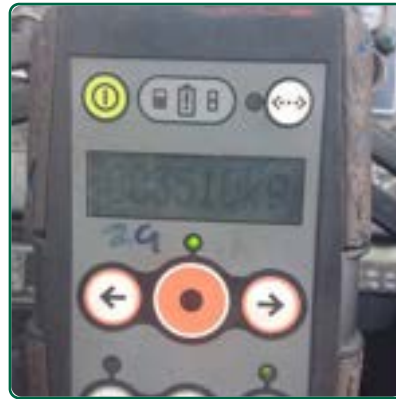
Rated Load - Boom Fully Extended - Load Measured
