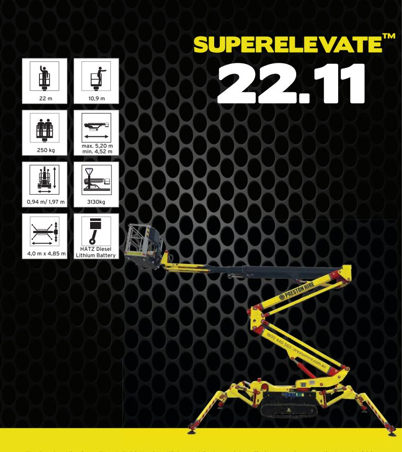
The Preston Hire SuperElevate<sup>™</sup> 22.11 spider lift is great for larger jobs, offering a maximum vertical reach of 22m, plus an outreach of 11m even with two people in the basket. Variable leg placement comes standard, enabling the unit to be set up in a number of configurations, the narrowest being a leg stance of only 1985mm, which is ideal when units are deployed in driveways, walkways or between buildings.
