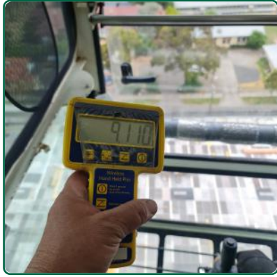
Dynamic Load Test
