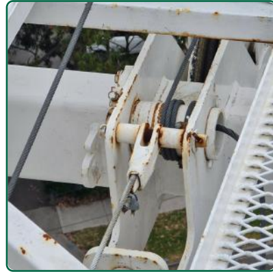
Correct Assembly and Connection of Trolley Rope Anchor
