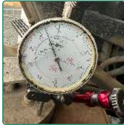
Articulation Joint .17mm measured as per Terex procedure. Allowable limit is .1mm. Suggest tightening articulation at next service.
