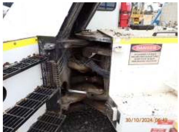
Photo 4: Boom articulation welds
